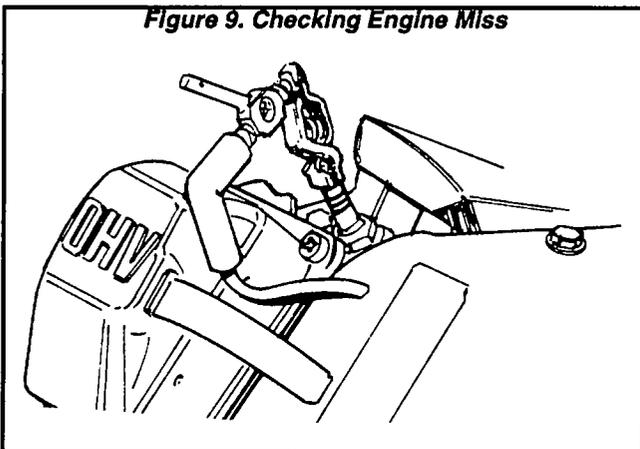
Figure 9. Checking Engine Miss
