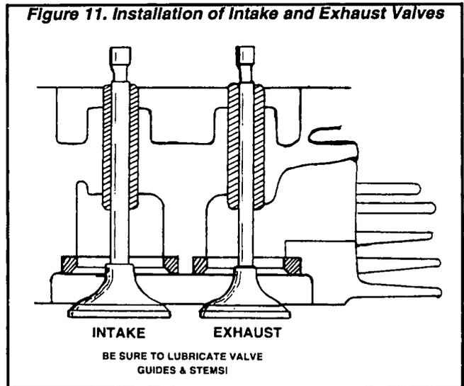
3. Install the valve spring washers, valve springs and valve spring retainers over the valve guides.
