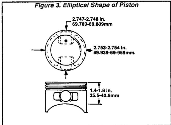
Figure 3. Elliptical Shape of Piston
