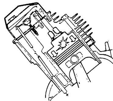
Figure 4. Exhaust Stroke
