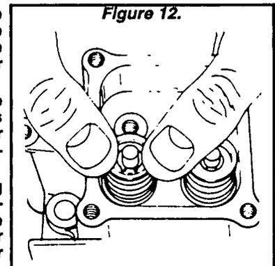
4. After both valves have been retained in the cylinder head, position a new head gasket and install the cylinder head.
