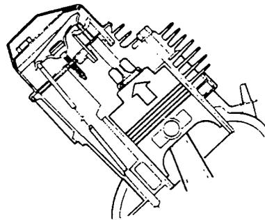
Figure 3. Power Stroke
