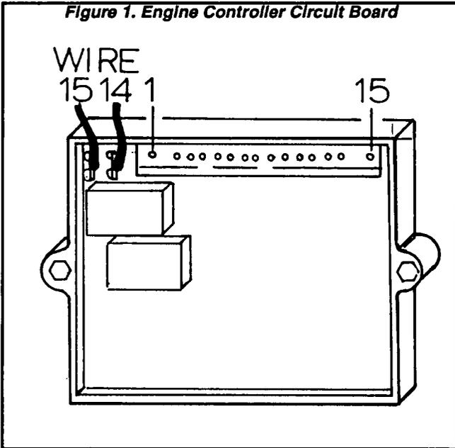
Figure 1. Engine Controller Circuit Board
