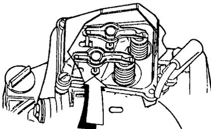
7. Install the push rod with either end against the tappet.
