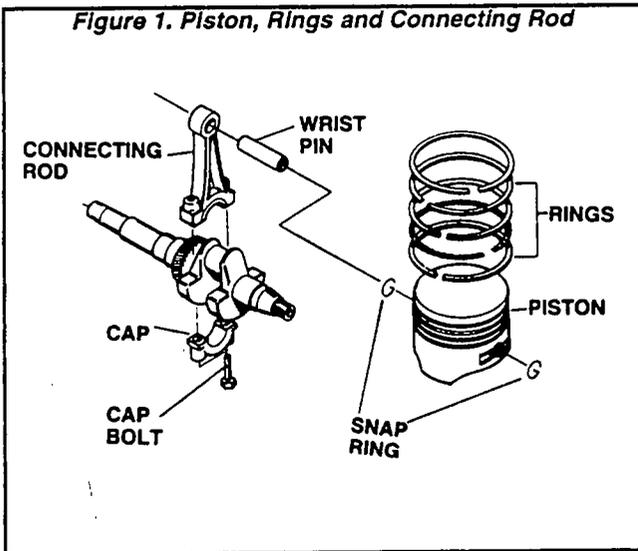
Figure 1. Piston, Rings and Connecting Rod
