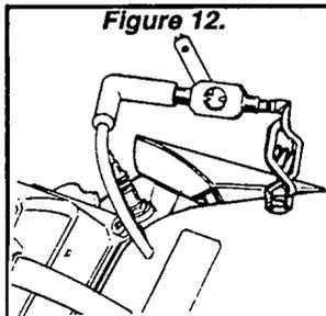
If sparking occurs with the **BROWN** wire grounded but did NOT occur under "TESTING FOR SPARK", the Ignition Sensor is probably defective and should be replaced.
