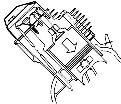
Figure 2. Compression Stroke
