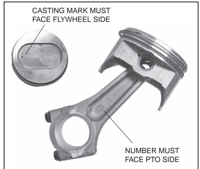
Figure 12-9. Assemble #2 Rod And Piston
