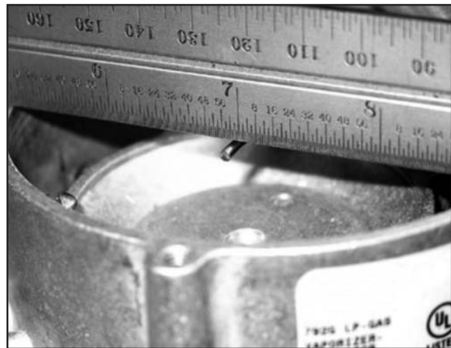
Figure 3-22. Make Sure Secondary Lever is Flush With Top of Casting
