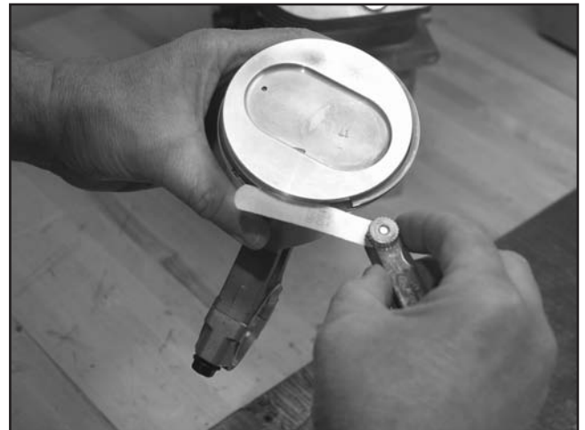
Figure 12-3. Check Ring Grooves
