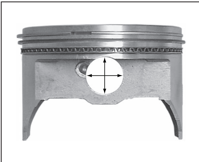
Figure 12-5. Check Piston Pin Bore
