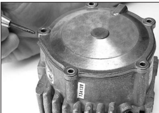
Figure 3-29. Install Secondary Cover
