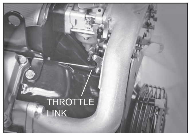
Figure 3-4. Horizontal Shaft Carburetor
