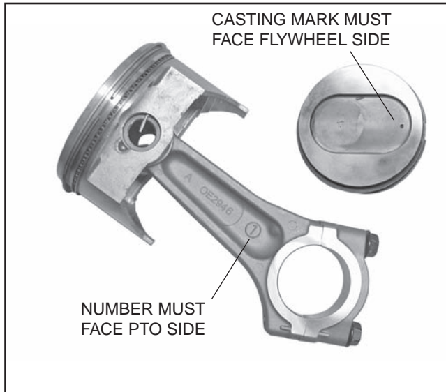
Figure 12-8. Assemble #1 Rod And Piston
