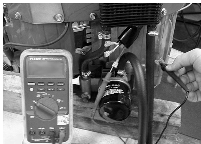
Figure 7-2. Testing DC Output Wire
