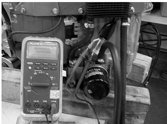
Figure 7-1. Testing AC Output
