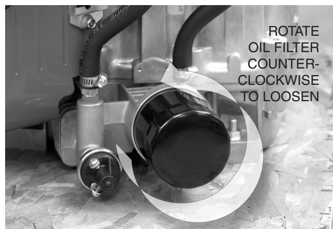
Figure 8-4. Removal of Oil Filter
