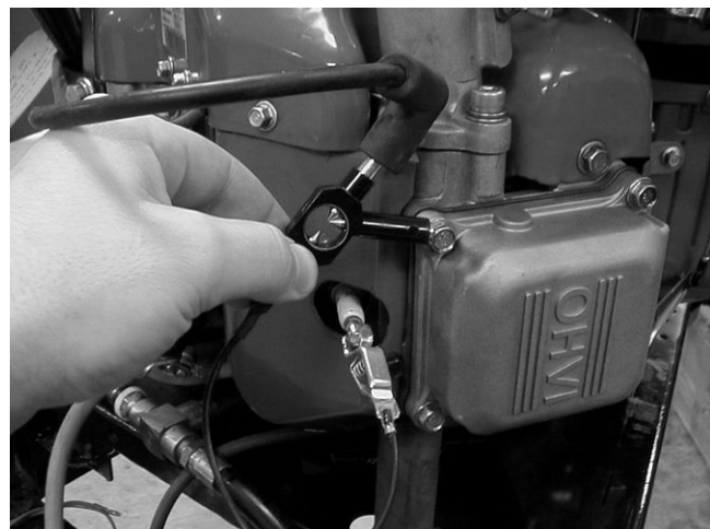
Figure 1-7. Checking For Fouled Plugs
