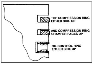
Figure 7. Ring Locations in Piston Grooves
