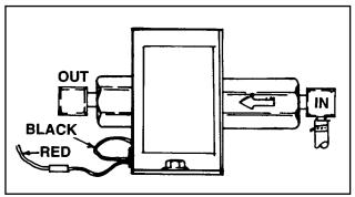
Figure 2. Electric Fuel Pump
