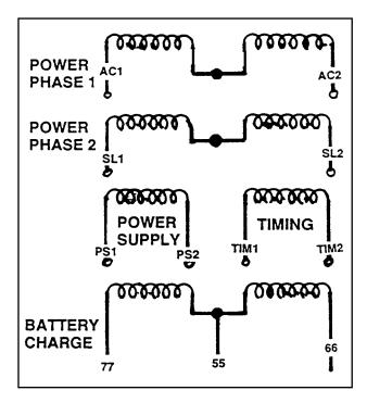
Figure 3. Schematic - Stator Windings
