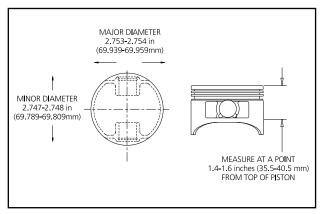
Figure 3. Elliptical Shape of Piston
