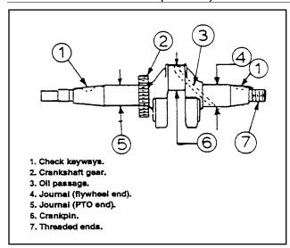
Figure 5. Points to Check on Crankshaft
