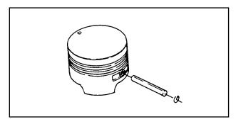
F figure 2. Piston Pin Removal
