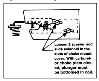
Figure 2. Choke Adjustment
