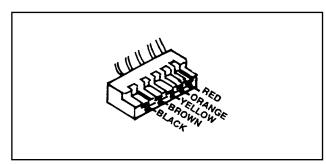
Figure 2. The Stepper Motor Connector
