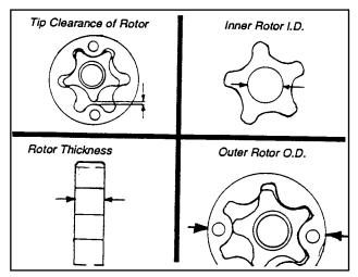
Figure 3. Oil Pump Check Points
