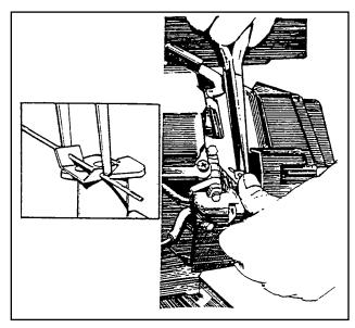
Figure 5. Adjusting Throttle Linkage
