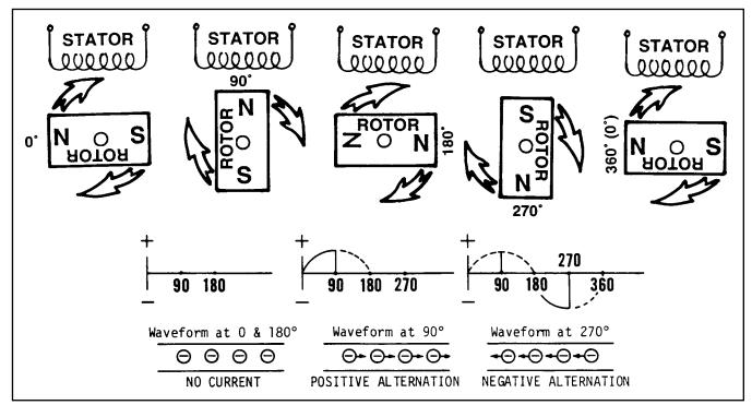
Figure 4. Operation of a Simple Generator
