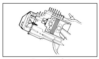
Figure 3. Power Stroke
