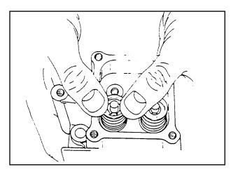
Figure 5. Removal of Valve Spring
