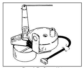
Figure 3. The Stepper Motor
