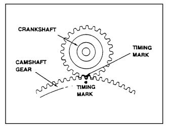
Figure 10. Alignment of Timing Marks
