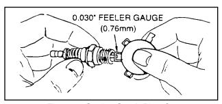
Figure 6. Setting Spark Plug Gap
