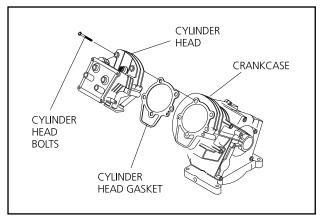
Figure 4. Cylinder Head Removal
