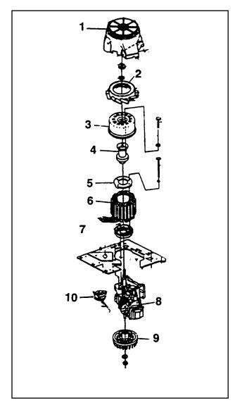
Figure 1. Exploded View of Generator Proper
