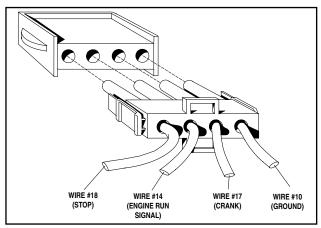
Figure 1. Remote Panel Plug-In Receptacle
