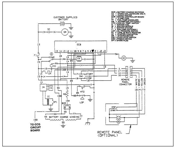
Figure 1. Schematic- Engine DC Control System
