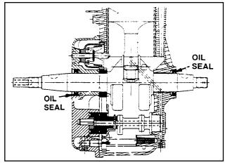
Figure 4. Crankshaft Oil Seals
