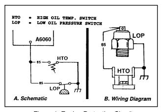
Figure 1. Engine Protective Circuit
