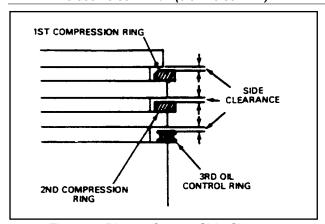
Figure 6. Ring to Groove Side Clearance
