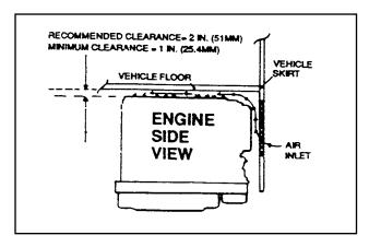
Figure 5 — Air Inlet in Vehicle Skirt
