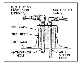
Figure 1. Sharing a Fuel Supply Tank
