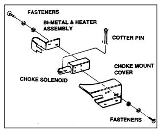
Figure 1. Choke Solenoid Parts
