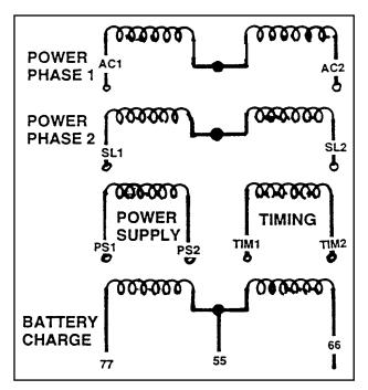
Figure 5. Schematic- Stator Windings
