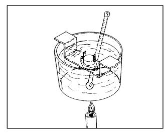
Figure 3. Testing the Oil Temperature Switch
