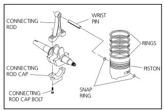
Figure 1. Piston, Rings and Connecting Rod
