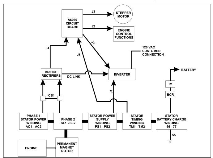
Figure 1. Block Diagram- A Generator System
