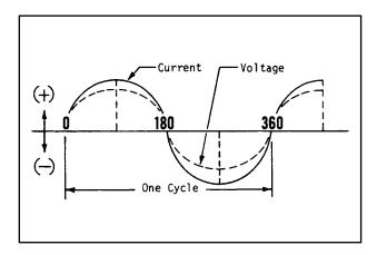
Figure 5. Alternating Current Sine Wave
