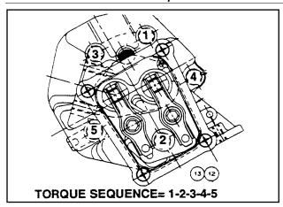
Figure 13. Head Bolts Tightening Sequence
