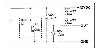
Figure 3. Ignition Sensor Schematic
