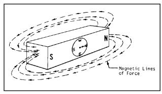
Figure 1. Magnetic Lines of Force
