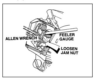
Figure 16. Adjusting Valve Clearance
