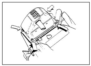
Figure 18. Rocker Arm Cover Installation
