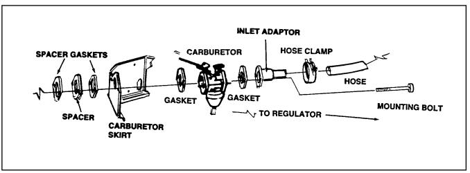
Figure 6. Carburetor Removal
