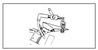
Figure 8. Testing for Spark
