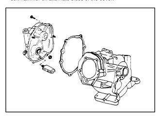
Figure 1. Crankcase Cover Removal
