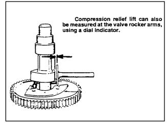
Figure 8. Measuring Compression Release Lift
