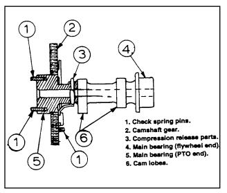
Figure 4. Points to Check on Camshaft
