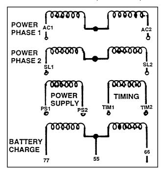
Figure 2. Schematic- Stator Windings
