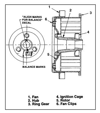
Figure 2 Permanent Magnet Rotor Assembly
