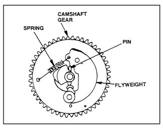
Figure 7. Compression Release Mechanism on Camshaft
