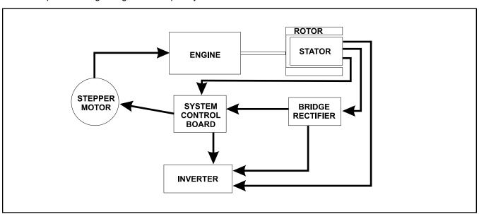
Figure 10. Block Diagram of the Impact 36 Plus System
