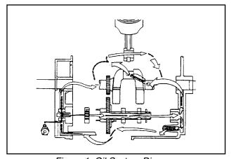
Figure 1. Oil System Diagram
