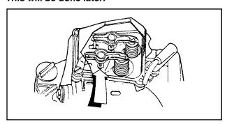
Figure 14. Install Rocker Arm & Pivot Ball stud
