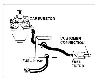
Figure 2. Typical Gasoline Fuel System
