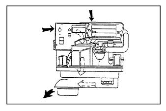
Figure 1 — Air Flow Through Engine-Generator
