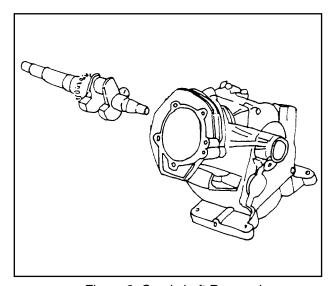
Figure 3. Crankshaft Removal
