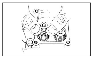
Figure 12. Installing Valve Spring Washers
