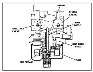
Figure 2. Carburetor Sectional View
