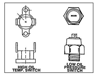
Figure 2. Engine Protective Devices
