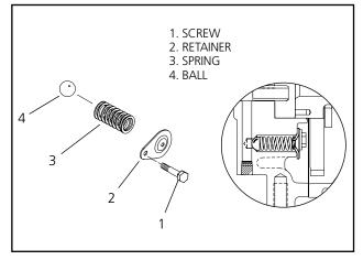
Figure 5. Oil Pressure Relief Valve
