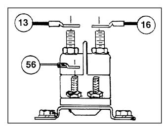
Figure 3. Starter Contactor
