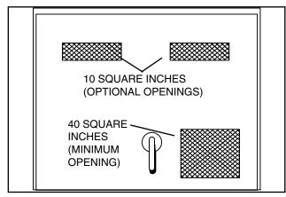
Figure 2 — Air Inlet in Compartment Door
