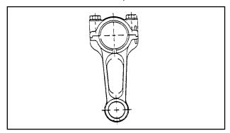
Figure 9. Connecting Rod
