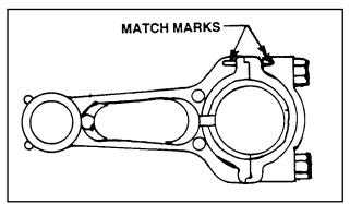
Figure 10. Match Marks on Rod and Cap
