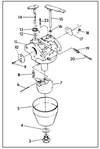
Figure 3. Carburetor Exploded View
