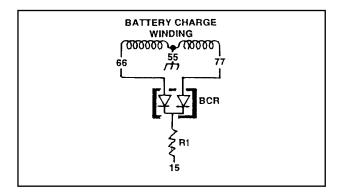
Figure 3. Battery Charge Windings and Rectifier
