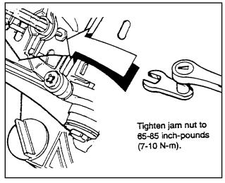
Figure 17. Tightening Pivot Ball Jam Nut
