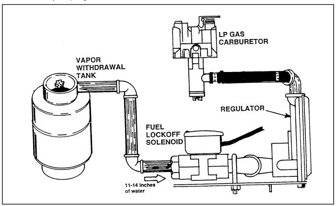
Figure 1. A Typical LP Gas Fuel System
