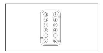
Figure 11. 12 Position Connector on Inverter
