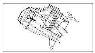
Figure 1. Intake Stroke
