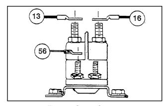
Figure 5. Starter Contactor
