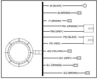
Figure 2. Stator Leads
