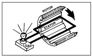
Figure 3. A Simple Revolving Field Generator
