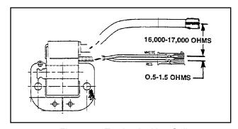
Figure 13. Testing Ignition Coil
