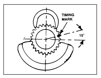
Figure 9. Timing Mark on Crankshaft Gear
