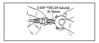
Figure 8. Checking Spark Plug Gap
