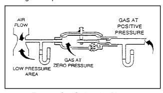
Figure 2. Gas Carburetion Diagram
