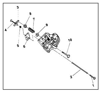
Figure 1. Valve Train Components
