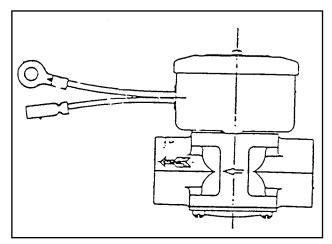
Figure 3. Fuel Lockoff Solenoid
