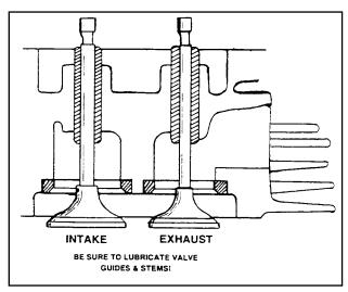
Figure 11. Installation of Intake and Exhaust Valves
