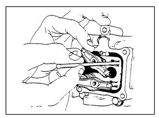
Figure 3. Rocker Arm, Push Rod & Guide Plate
