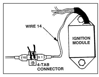
Figure 9. Ignition Module & 4-Tab Connector
