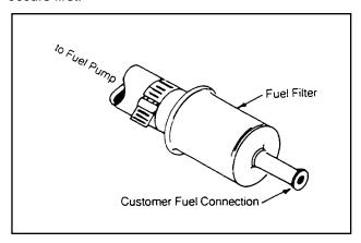
Figure 1. Fuel Filter (Typical)
