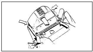
Figure 2. Removal of Rocker Arm over
