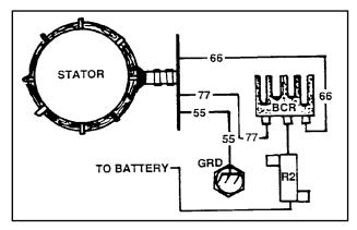
Figure 4. Battery Charge Circuit
