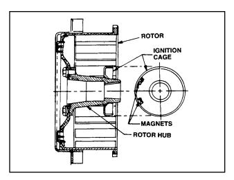
Figure 1. Ignition Cage Assembly
