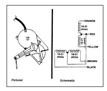
Figure 3. The Stepper Motor
