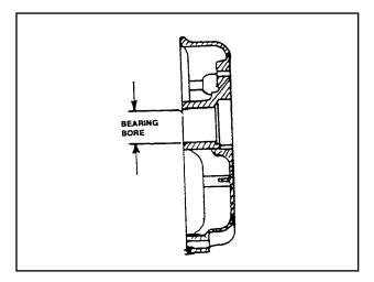
Figure 6. Bearing Bore in Crankcase Cover
