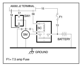
Figure 1. Schematic - Cranking Circuit
