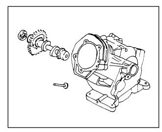
Figure 2. Camshaft Removal
