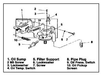
Figure 7. Oil Filter Support
