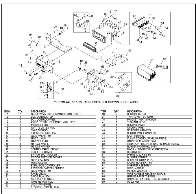
Figure 1. Exploded View of Control Panel
