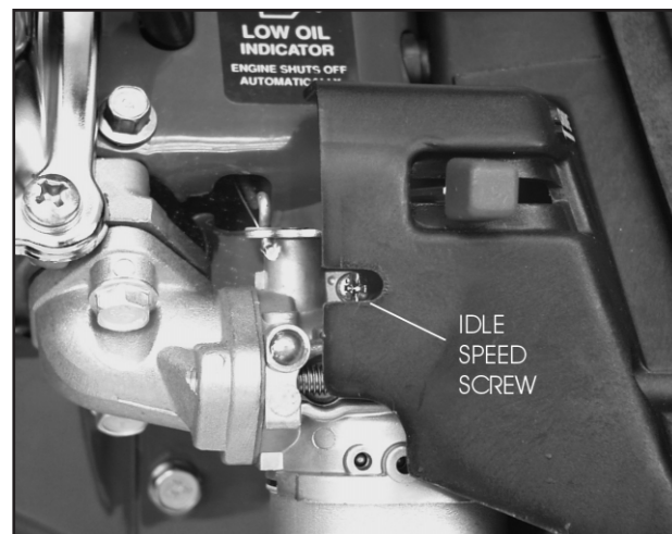
Figure 3.6 — Carburetor Adjustment (Typical)
