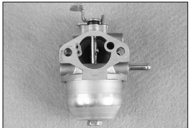
Figure 2.5 — Typical Carburetor with Choke
