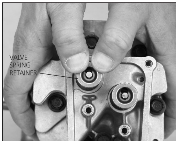
Figure 9.12 — Compressing Valve Spring
