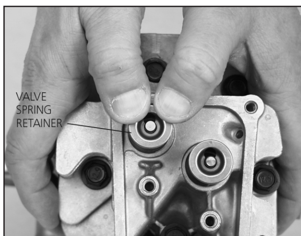
Figure 9.5 — Compressing Valve Springs
