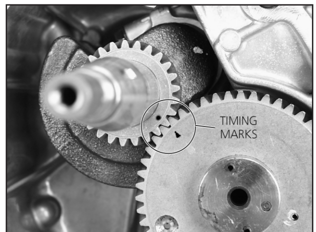
Figure 11.11 — Alignment of Timing Marks
