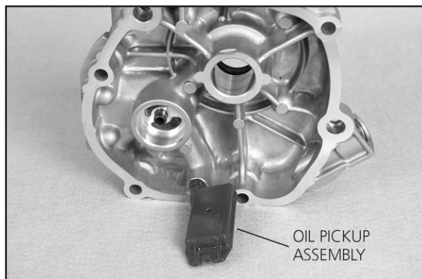
Figure 12.2 — Oil Pickup Assembly
