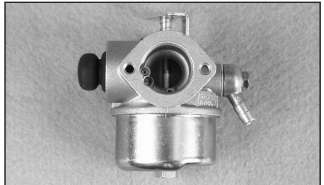
Figure 2.4 — Typical Carburetor with Primer
